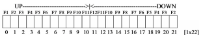
Figure 4 - Solution encoding for a twelve storey building corresponding to one car of the group and its associated physical button box.
