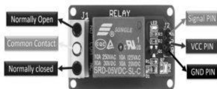
Relay is one kind of electro-mechanical component that functions as a switch. The relay coil is energized by DC so that contact switches can be opened or closed. A single channel 5V relay module generally includes a coil, and two contacts like normally open (NO) and normally closed (NC).
