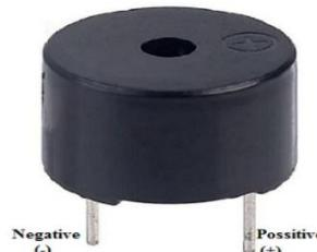
An audio signaling device like a beeper or buzzer may be electromechanical or piezoelectric or mechanical type. The main function of this is to convert the signal from audio to sound. Generally, it is powered through DC voltage and used in timers, alarm devices, printers, alarms, computers, etc. Based on the various designs, it can generate sounds like alarm, music, bell and siren.
