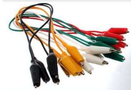
A jump wire is an electrical wire, or group of them in a cable, with a connector or pin at each end, which is normally used to interconnect the components of a breadboard or other prototype or test circuit, internally or with other equipment or components of a breadboard or other prototype or test circuit, internally or with other equipment or components, without soldering.
